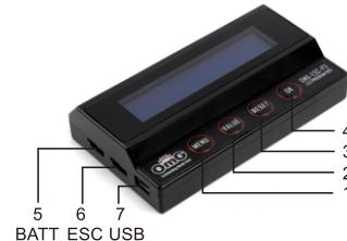
1. MENU: circularly switch programming projects and modes; Exit the user-defined parameters setting; Enter the programming project setting.
